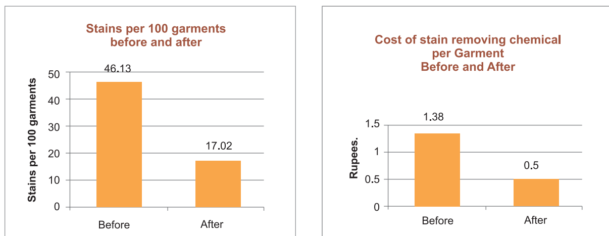
Figure 3.4- Graphs Showing Reduction in Stains per hundred garment and reduction in cost of stain removing chemical after the implementation of QIP
